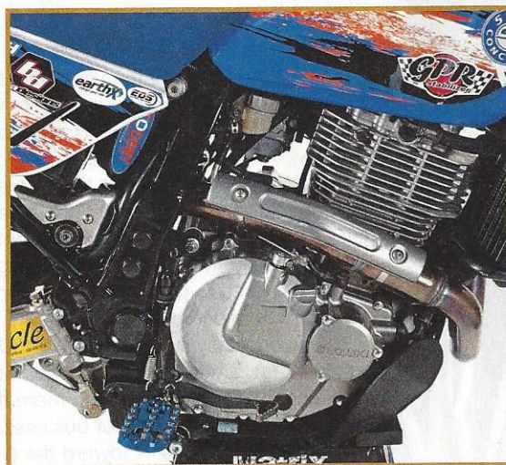
The DR motor got a big-bore kit and a Mikuni pumper carb, resulting in crazy-low-rpm torque.
