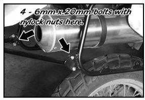
10. Once all of the hardware is in place, please tighten the four bolts on the right rack first, then the four bolts on the left rack and then the four bolts that hold the crossbar in place.
